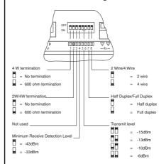
Modem parameters are adjusted via the DIL switch as shown above.
