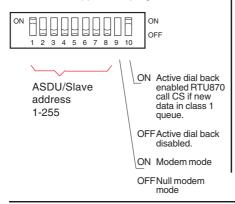
The logical common ASDU address is defined as the sum of the binary value selected using switch 1-8 and the binary value of the logical address configured in the FLASH (default = 0).
