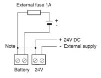
Battery: An external fuse 1A must be mounted
