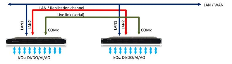
Two communication links are used for data replication and status monitoring in order to withstand *One point of failure*.
