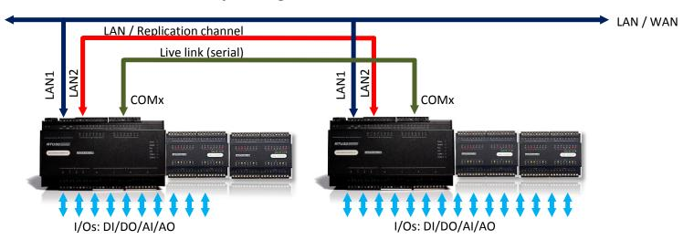
Two communication links are used for data replication and status monitoring in order to withstand *One point of failure*.
