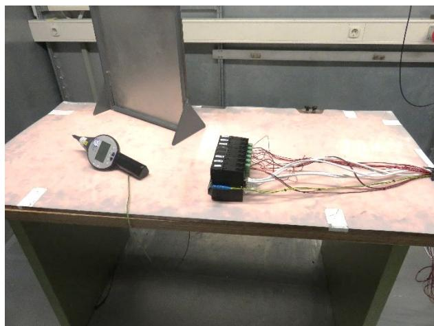
Fig. 4-1: Test setup for ESD testing
