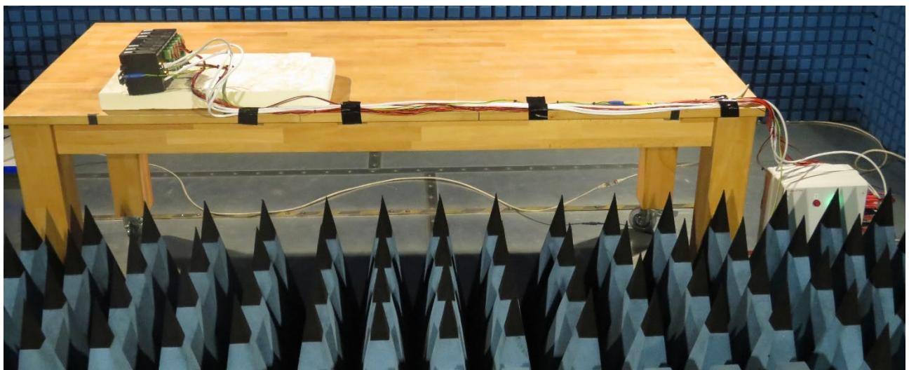
Fig. 4-4: Test setup for radiated susceptibility test (left side)
