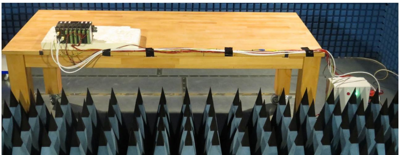
Fig. 4-3: Test setup for radiated susceptibility test (front side)
