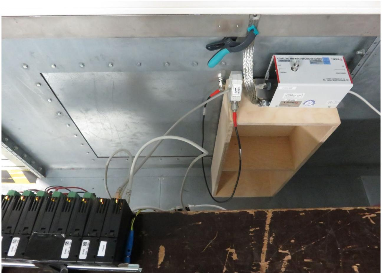
Fig. 3-3: Test setup for the disturbing current measurement
