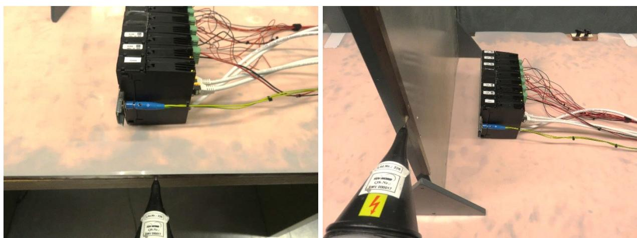
Fig. 4-2: Test setup for indirect ESD testing (CD on coupling planes, exemplary)
