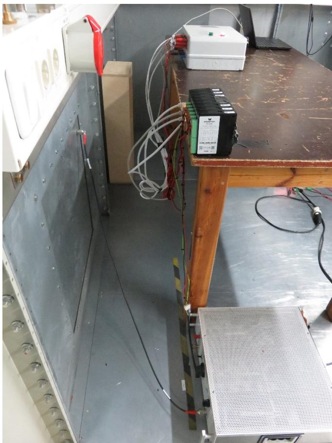
Fig. 3-1: Test setup for the disturbing voltage measurement
