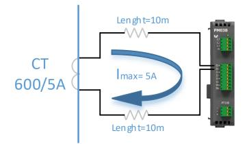
Burden( $\Omega$ ) = (2 × R<sub>cable</sub>) + R<sub>module</sub> = 2×(10×0.0115) + 0.022 = 0.252  $\Omega$
