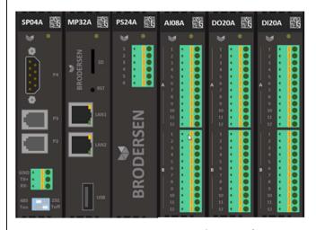
Figure 3: MP32A hardware interface with I/O
