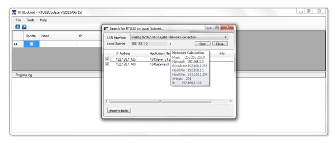
Select the relevant LAN Interface on your PC – use default if you only have one. Check that the local subnet is correct and press "Start" to search for RTUs. If the RTUs are assigned a correct IP address and connected to your network, they will appear in the list as shown above. You can now use the check box at the left side and the "Insert to table" button to copy the found RTUs to your table in the Main window.
