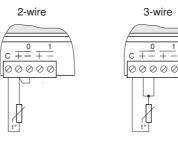
Sensor cable length above 30m is not recommended. If cable length is more than 5m 3-wire sensors are recommended to avoid offset i naccuracy caused by loss in cables.
