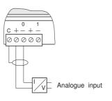
**Analogue input** (Pt-100 sensor input) 1 Pt-100 sensor input. Is configured from the factory. Standard range -50-100°C. 2 or 3 wire is supported.
