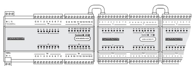
If the current consumption of the expansion modules exceeds the capability of the power supply, an additional power supply must be inserted.
